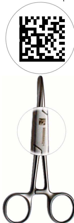
Figure 3) HIBC Unique Identification Mark (UIM) applied to a surgical instrument (UIM enlarged)
