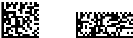
Figure 1) Datamatrix square format 16x16 versus rectangular format 12x26
