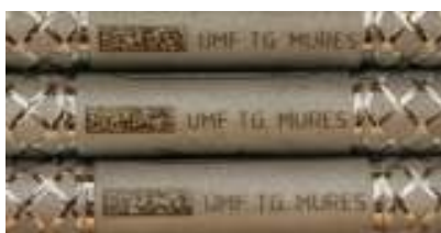
Bild 12) UIM on a round instrument as rectangular Data Matrix
