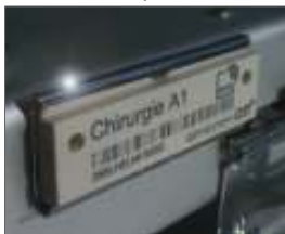
Fig. 8) Container plate and Code 128
